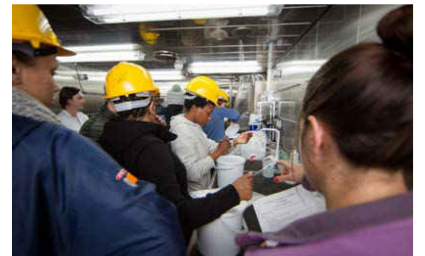
Students working on SEAmester II conduct an assignment on microplastics. The goal was to sample plastic in sand from Muizenberg beach. The students add water to the sand, stir vigorously, then allow the sample to settle. Plastic particles mixed in with the sand float to the surface of the water, where they can be collected and further analysed. Morgan Trimble
